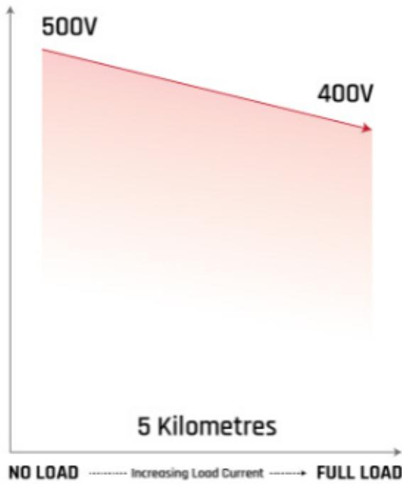
Voltage drop is the decrease of electrical voltage as current flows within an electrical circuit. The drop leads to a lower voltage at the endpoint. When current passes through an electrical circuit, a voltage drop occurs due to the resistance or impedance to the flow of the current.
